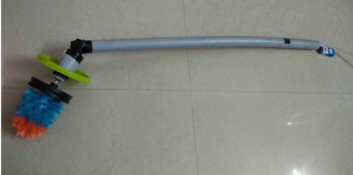
**It is made up of one metre plastic pipe. At one end motor with toilet brush is attached to clean with water spraying. On another end the controlling switch is fixed. It functions with the help of 9 volts battery power.**
