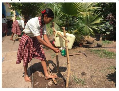
Siddhi has developed a hand washing device from trash. It requires three wooden sticks to create a frame, one more wooden stick to act as a foot lever, a plastic can as a water storage device, and some ropes, wires for tying.
